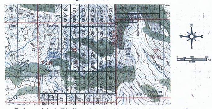
The above map depicts the SPS - 41 Lode mining claim, which is located in Section(s) \_\_ North, Range \_\_15 East. Gila and Salt River Baseline and Meridian, Gila County, Arizona. The claim corners, end centers and Location monuments are marked by 2 inch by 2 inch by 5 foot wooden post with aluminum tags. The bearings and distances between claims and tie point are depicted on the map.
