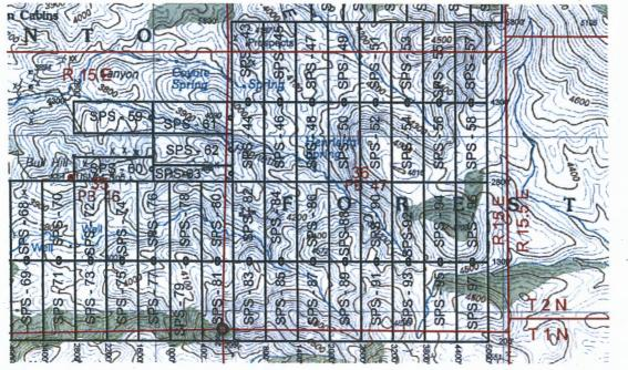
The above map depicts the SPS - 53 Lode mining claim, which is located in Section(s) North, Range 15 East. Gila and Salt River Baseline and Meridian, Gila County, Arizona. The claim corners, end centers and Location monuments are marked by 2 inch by 2 inch by 5 foot wooden post with aluminum tags. The bearings and distances between claims and tie point are depicted on the map.
