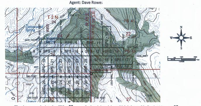
The above map depicts the SPS - 28 Lode mining claim, which is located in Section(s) \_\_\_\_\_\_\_ 2 North, Range \_\_\_\_\_\_ 15 East. Gila and Salt River Baseline and Meridian, Gila County, Arizona. The claim corners, end centers and Location monuments are marked by 2 inch by 2 inch by 5 foot wooden post with aluminum tags. The bearings and distances between claims and tie point are depicted on the map.
