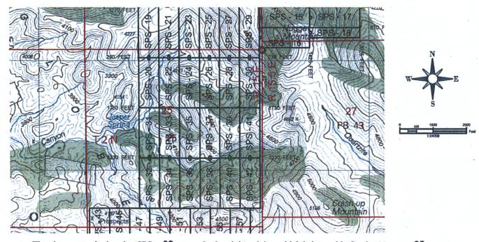
The above map depicts the SPS - 39 Lode mining claim, which is located in Section(s) \_\_\_\_\_\_ 25 Township \_\_\_\_\_ 2 North, Range \_\_\_\_\_ 15 East. Gila and Salt River Baseline and Meridian, Gila County, Arizona. The claim corners, end centers and Location monuments are marked by 2 inch by 2 inch by 5 foot wooden post with aluminum tags. The bearings and distances between claims and tie point are depicted on the map.
