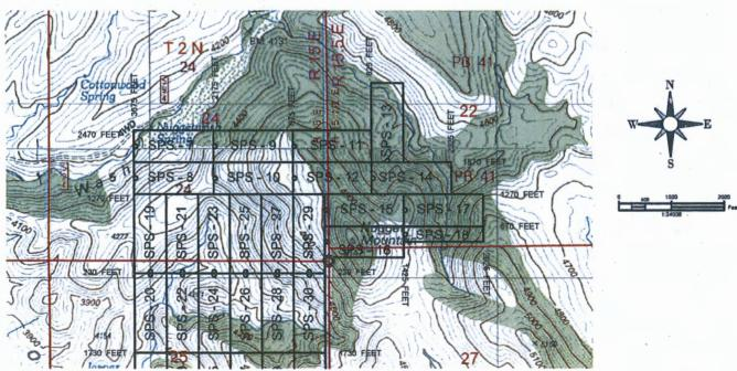
The above map depicts the SPS 12 Lode mining claim, which is located in Section(s) North, Range \_\_\_\_\_15 / 15.5 East. Gila and Salt River Baseline and Meridian, Gila County, Arizona. The claim corners, end centers and Location monuments are marked by 2 inch by 2 inch by 5 foot wooden post with aluminum tags. The bearings and distances between claims and tie point are depicted on the map.
