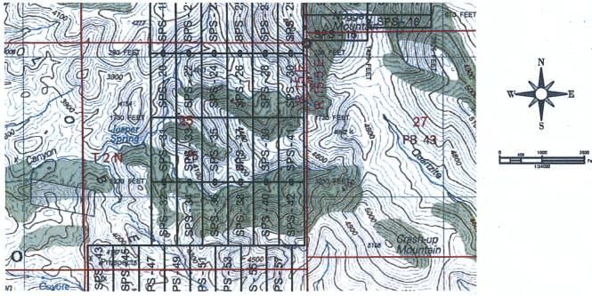
The above map depicts the SPS - 42 Lode mining claim, which is located in Section(s) \_\_\_\_\_\_\_ 2 \_\_\_\_\_ North, Range \_\_\_\_\_\_ 15 East. Gila and Salt River Baseline and Meridian, Gila County, Arizona. The claim corners, end centers and Location monuments are marked by 2 inch by 2 inch by 5 foot wooden post with aluminum tags. The bearings and distances between claims and tie point are depicted on the map.
