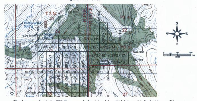
The above map depicts the SPS 8 Lode mining claim, which is located in Section(s) North, Range \_\_\_\_15 \_\_\_ East. Gila and Salt River Baseline and Meridian, Gila County, Arizona. 2 The claim corners, end centers and Location monuments are marked by 2 inch by 2 inch by 5 foot wooden post with aluminum tags. The bearings and distances between claims and tie point are depicted on the map.
