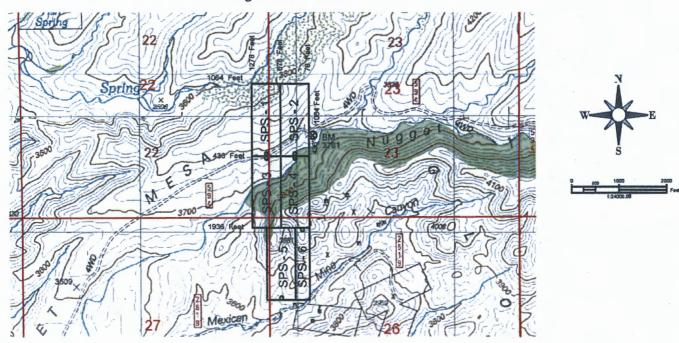
The above map depicts the SPS - 2 Lode mining claim, which is located in Section(s) North, Range 15 East. Gila and Salt River Baseline and Meridian, Gila County, Arizona. The claim corners, end centers and Location monuments are marked by 2 inch by 2 inch by 5 foot wooden post with aluminum tags. The bearings and distances between claims and tie point are depicted on the map.
