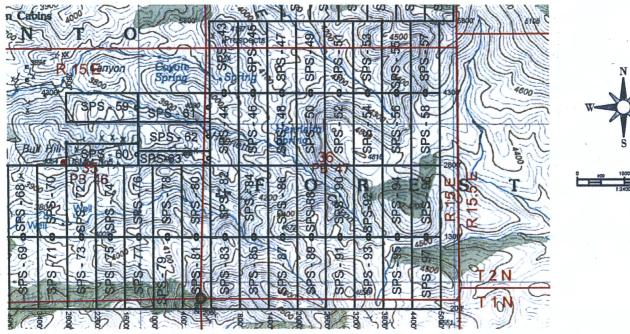
Lode mining claim, which is located in Section(s) The above map depicts the SPS - 43 North, Range 15 East. Gila and Salt River Baseline and Meridian, Gila County, Arizona. The claim corners, end centers and Location monuments are marked by 2 inch by 2 inch by 5 foot wooden post with aluminum tags. The bearings and distances between claims and tie point are depicted on the map.
